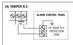
The tamper switch is Normally Closed while the keypad is secured on gang box. It is open when the keypad is removed from the gang box. To prevent sabotage, connect these terminals in series with a 24 hour N.C. protection zone of an alarm system if required.
