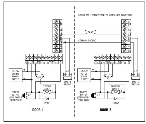
An inter-lock system needs two door controllers. This application example uses two of DC60SS, DC50SS or DC50FS with simple cross wire connection on their "Output 1 Inhibit" and "Inter-lock Control Output" terminals. It is necessary to link up the "(-) GND" terminals of the two keypads as common ground to achieve the inter-lock logical functions.
